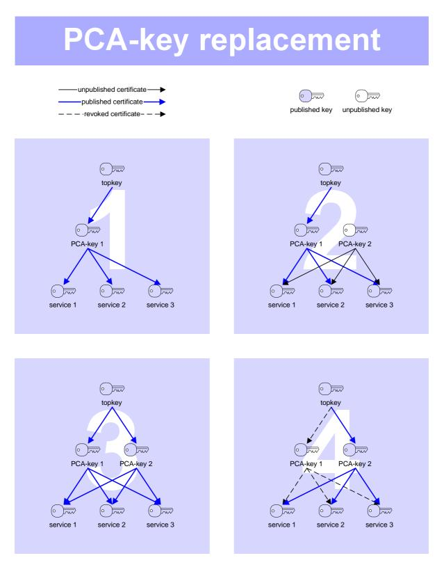
Step 1 shows the certification hierarchy in its basic (normal) state. No backup system is deployed. The two upper keys (top key and PCA key 1) are the supervisory authority's keys, while the keys beneath them are those of three certification service providers.
