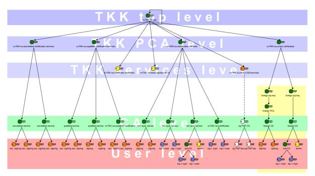
Telekom-Control GmbH, 31.10.2000 Entwurf einer TKK-Zertifizierungshierarchie – Draft of a TKK certification hierarch The top key of the supervisory authority, as well as its predecessors and successors, is the only key located at the uppermost level (TKK top level).
