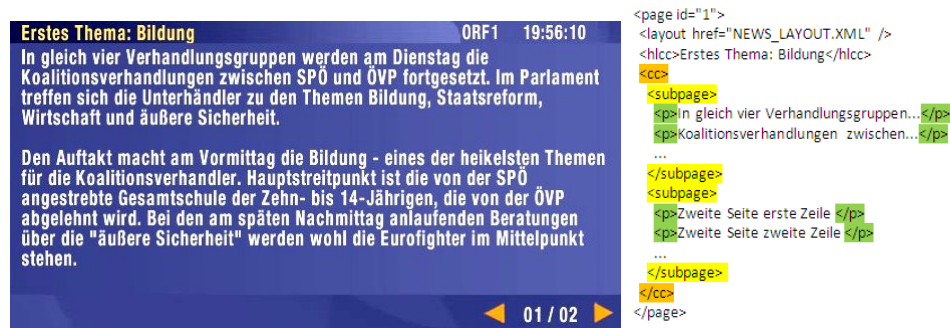
© ORF 2008 Figure 8: Content Container with its XML structure
