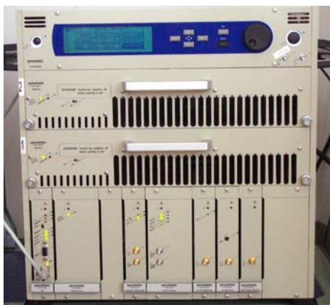
Figure 36: DVB-T transmitter and antenna at the Institute of Communication Networks and Satellite Communications
