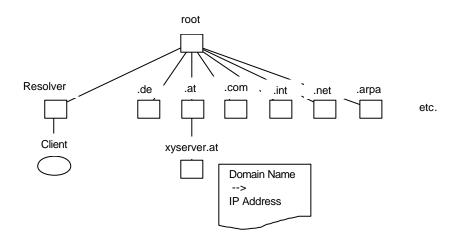
In practice, a request for the IP address of a web page (e.g., http://www.rtr.at) is handled by a local DNS server, which sends a request to the root server and receives the IP address of the DNS server for the ".at" zone, to which the request is then forwarded. This strictly hierarchical procedure repeats itself until the request has been sent to the server which can provide the correct IP address for http://www.rtr.at.
